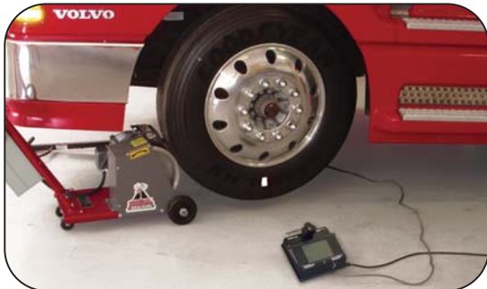
1. A spinner brings the wheel up to speed.
