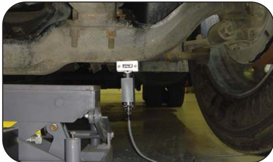
2. A sensor measures wheel vibration
