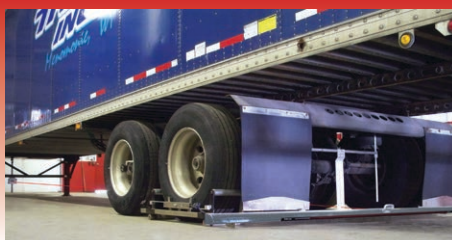
Figure C - With the Bee Line Laser Tandem Aligner, offset axles and axles with uneven spacers are set perfectly at 90° to the centerline of the vehicle. Additional axles are then simply set with a tram gauge.
