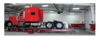
The longer design of the Space Saver lifting ramp creates a more gradual incline and requires less runway sections.
