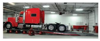
With the truck in position, Runways are hydraulically lifted with the touch of a button.
