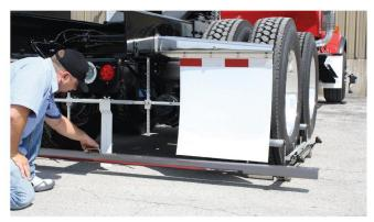
Our 22000 Rear axle aligner gauges tractor and trailer axles in their operating position and records live readings during corrections. All axles are set perfectly perpendicular to the centerline of the chassis.axles are set perfectly perpendicular to the centerline of the chassis.
