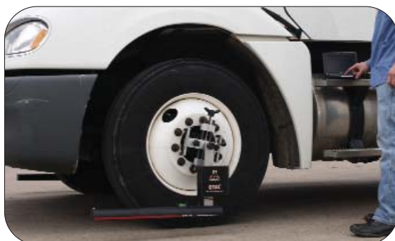
A technician can take the alignment check to the truck and get a live toe reading in minutes.
