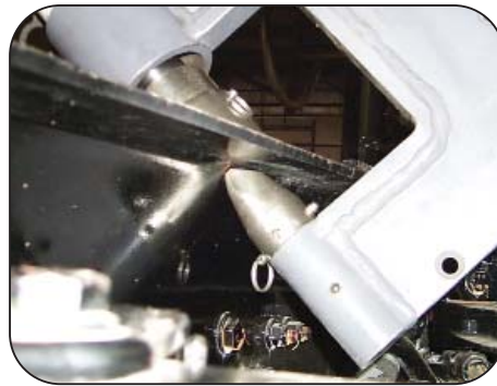
WITH THE CHISEL (LEFT) AND THE LOWER ANGLE PAD (RIGHT), CORRECTIONS CAN EASILY BE MADE TO THE RADIUS EDGE BETWEEN THE WEB AND FLANGE.
