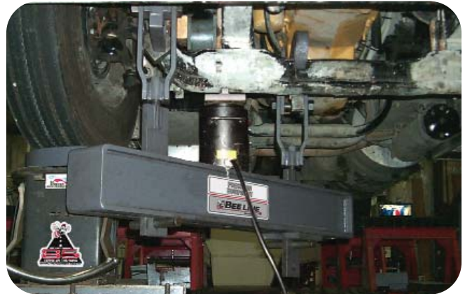
Caster twist correction setup.
