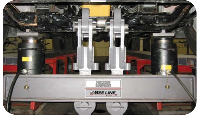
Negative Camber Correction on both sides.
