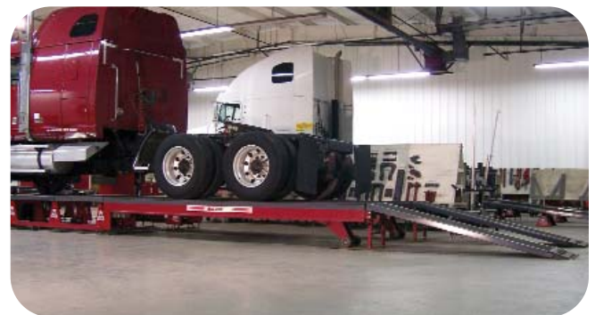
With the truck in position, the Runways are hydraulically lifted with the touch of a button.
