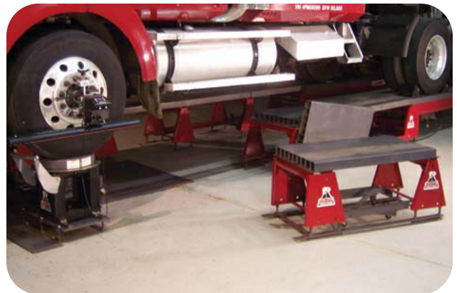
The forward runways are removable for easy access to the vehicle when making a variety of adjustments.
