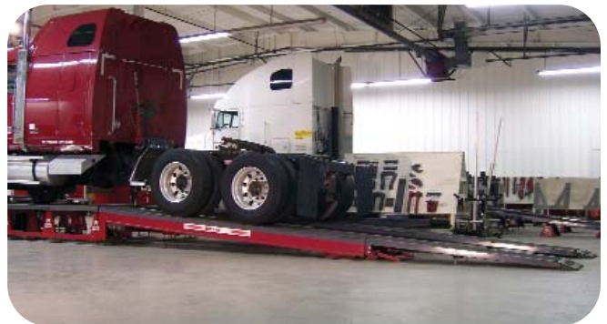
The longer design of the new Space Saver lifting ramp creates a more gradual incline and requires less runway sections.
